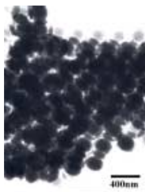
Figure 5 TEM image of Pd nanoparticles formed around the PSA spheres
