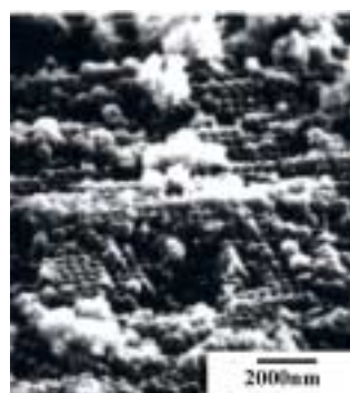
Figure 2 The Au formed around the PSA spheres in the template
